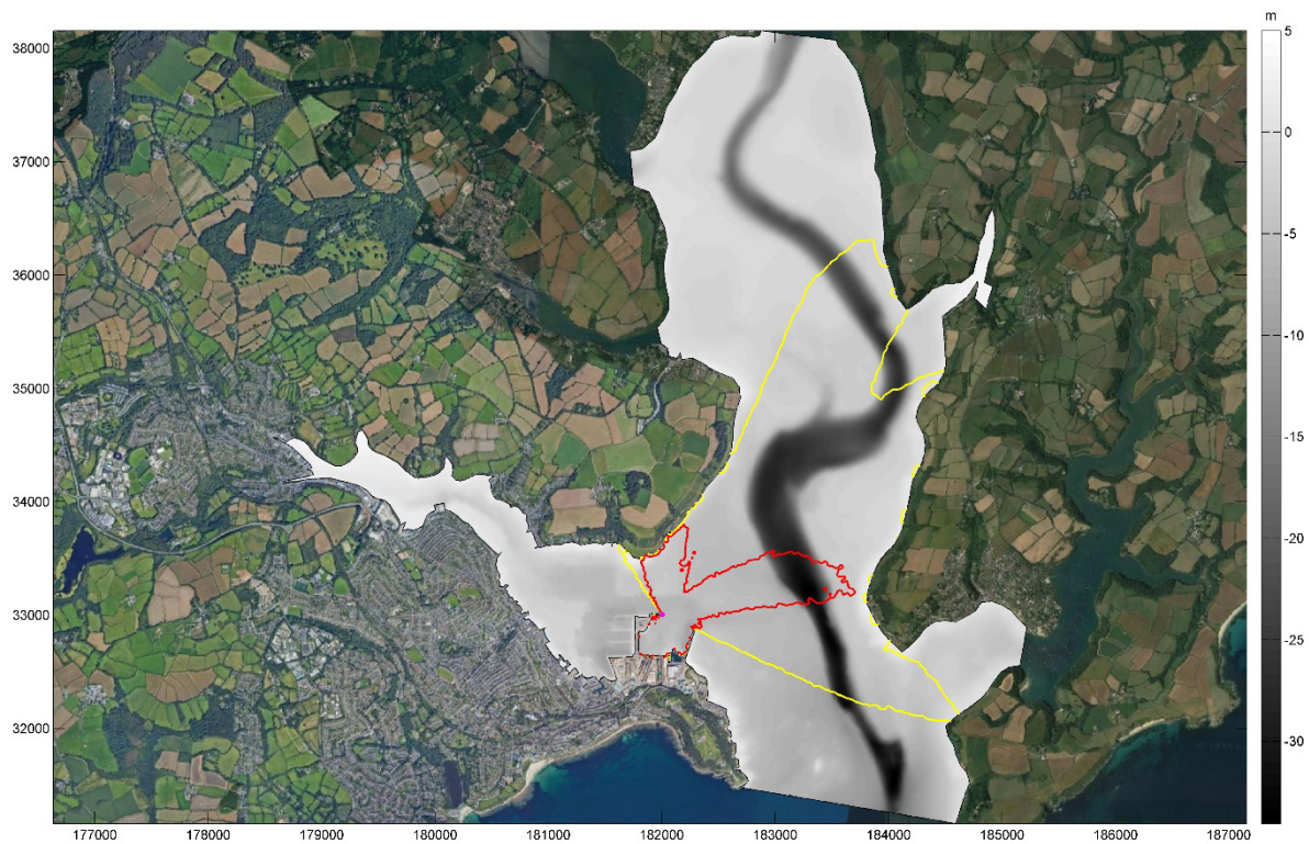
Figure 7.4: Predicted SEL cum impact footprint for the very high frequency cetacean hearing group for demolition with a hydraulic hammer at the Northern Arm (Location 1)
