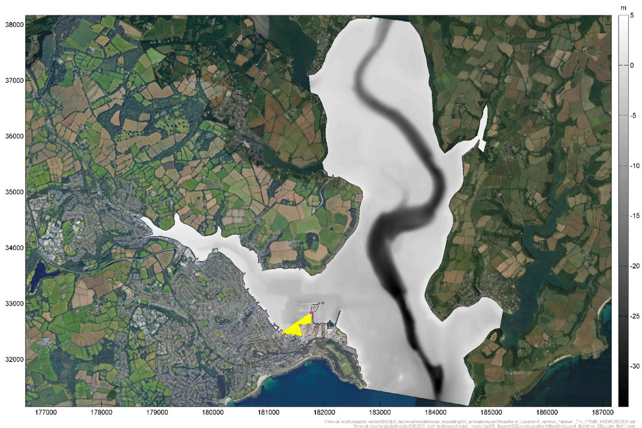
Figure 7.41: Predicted SEL cum impact footprint for the very high frequency cetacean hearing group for dredging with a backhoe at the FLOW deck (Location 4)
