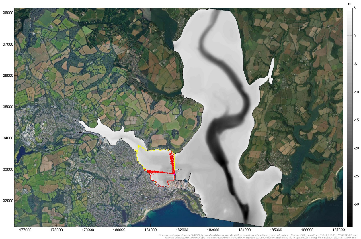
Figure 7.47: Predicted SEL cum impact footprint pinnipeds for percussive piling, with a soft start procedure, at the FLOW Deck (Location 4)
