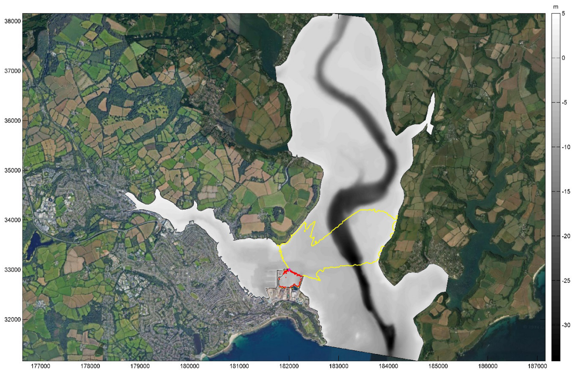
Figure 7.5: Predicted SEL_{cum} impact footprint for pinnipeds for demolition with a hydraulic hammer at the Northern Arm (Location 1)
