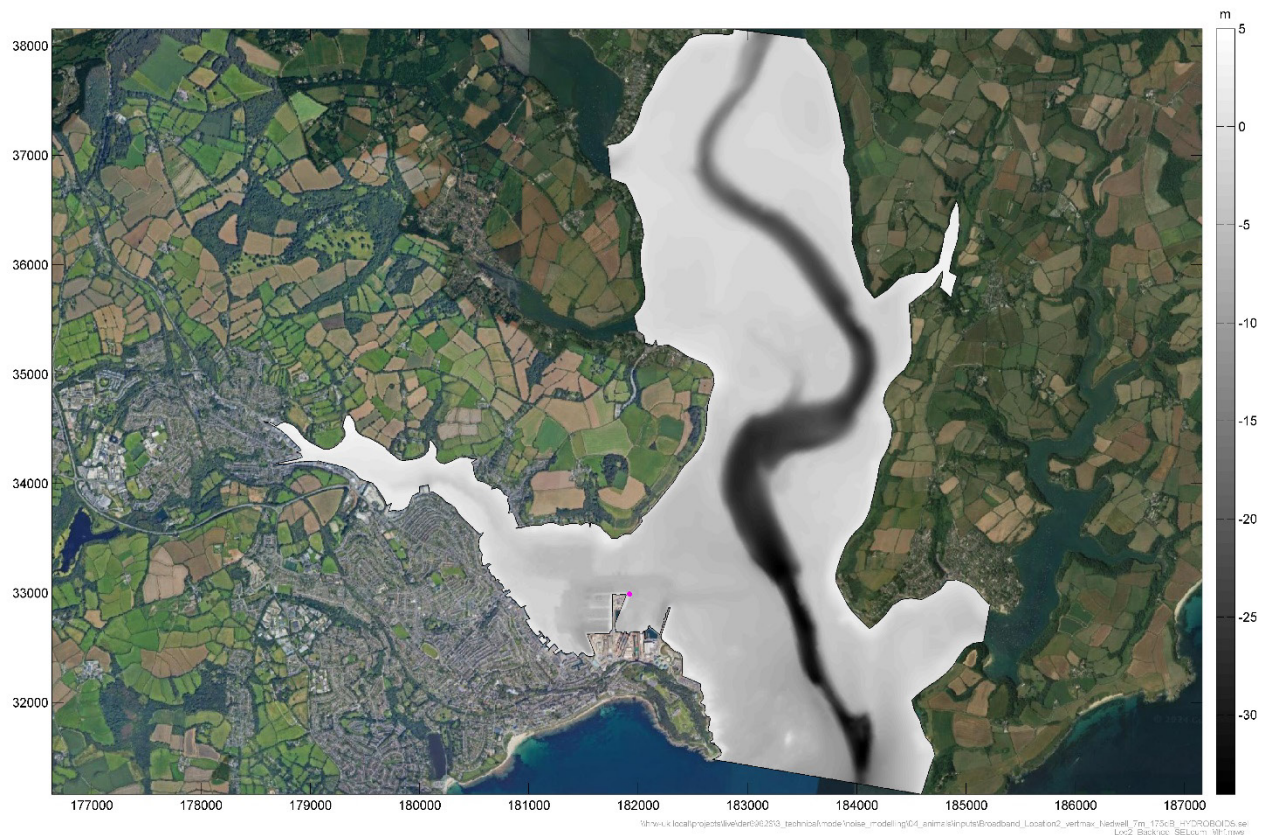
Figure A.7: Predicted SEL_{cum} impact footprint for the for high frequency cetaceans for dredging at Western Wharf (Location 2)
