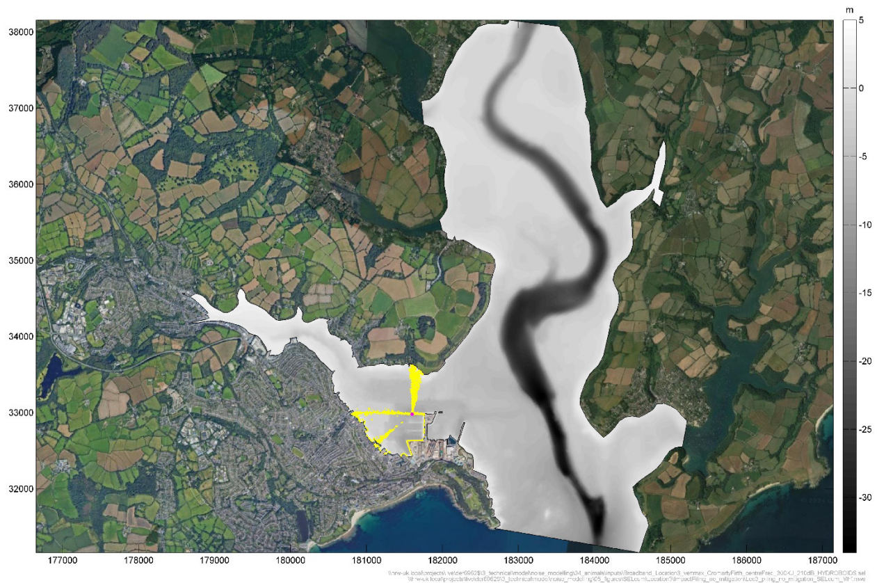
Figure A.23: Predicted SEL cum impact footprint for the for high frequency cetaceans for pile driving at Queen's Wharf (Location 3)
