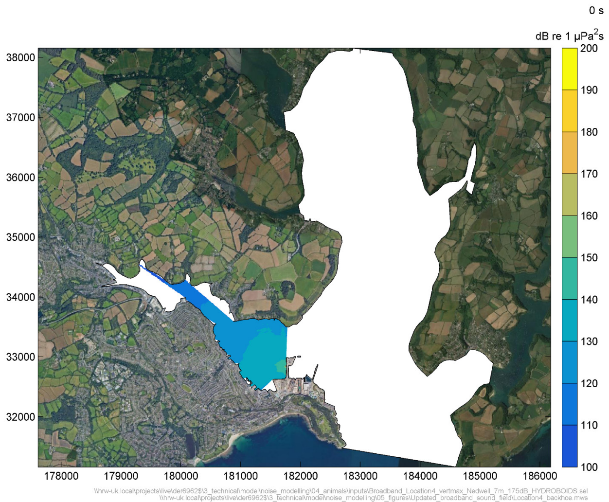
Figure 7.40: Predicted single strike SEL sound field for backhoe dredging at Location 4
