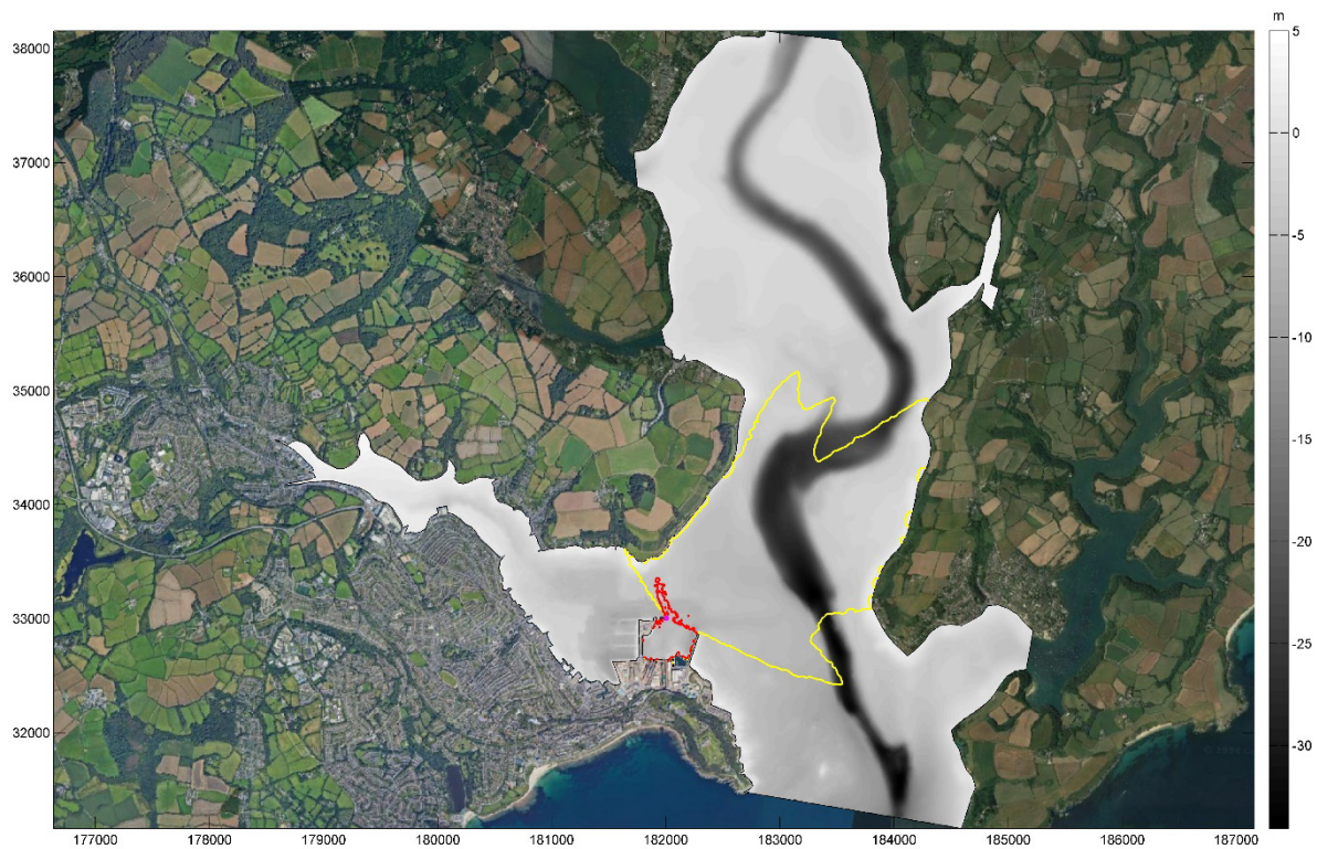
Figure 7.2: Predicted SEL cum impact footprint for the low frequency cetacean hearing group for demolition with a hydraulic hammer at the Northern Arm (Location 1)
