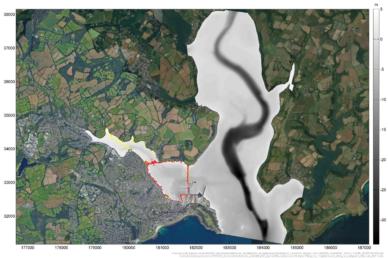
Figure 7.46: Predicted SEL_{cum} impact footprint for the very high frequency cetacean hearing group percussive piling, with a soft start procedure, at the FLOW Deck (Location 4)
