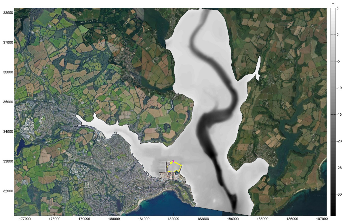
Figure 7.3: Predicted SEL_{cum} impact footprint for the high frequency cetacean hearing group for demolition with a hydraulic hammer at the Northern Arm (Location 1)
