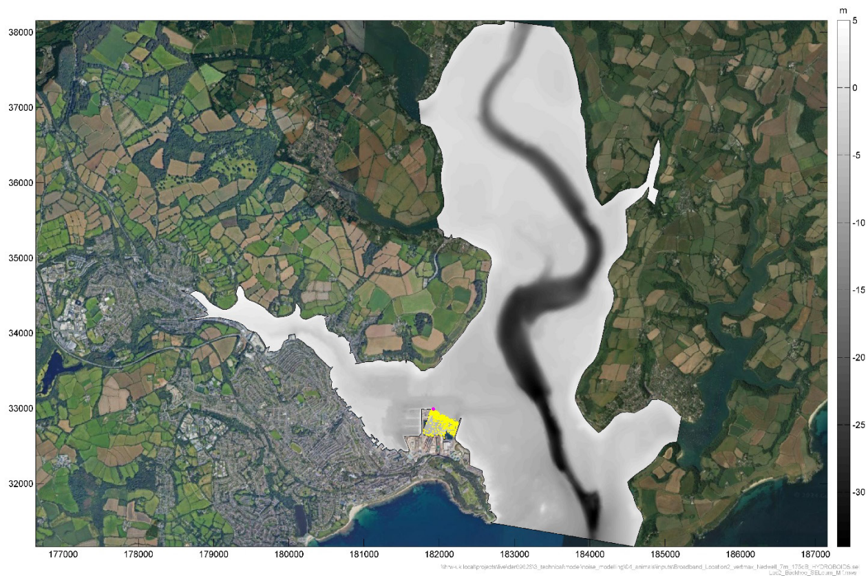
Figure A.8: Predicted SEL_{cum} impact footprint for the for low frequency cetaceans for dredging at Western Wharf (Location 2)
