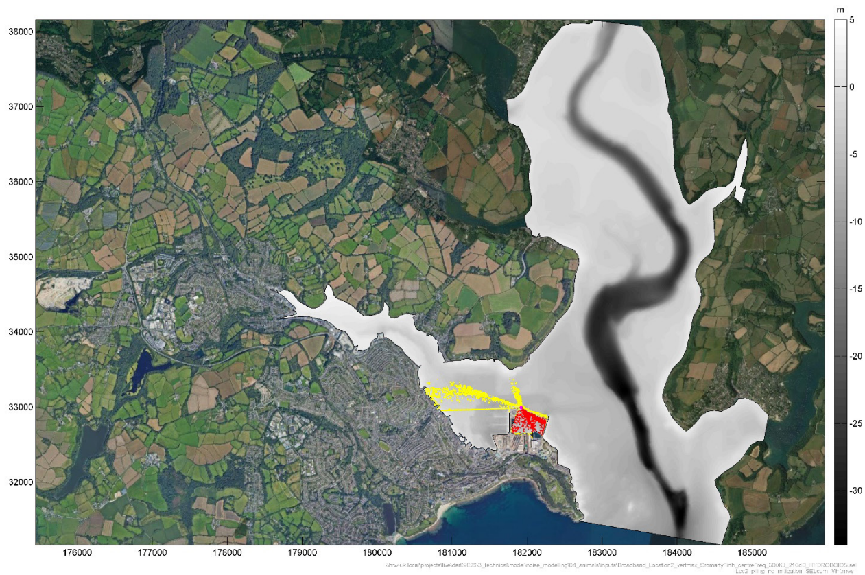
Figure A.11: Predicted SEL cum impact footprint for the for high frequency cetaceans for pile driving at Western Wharf (Location 2)
