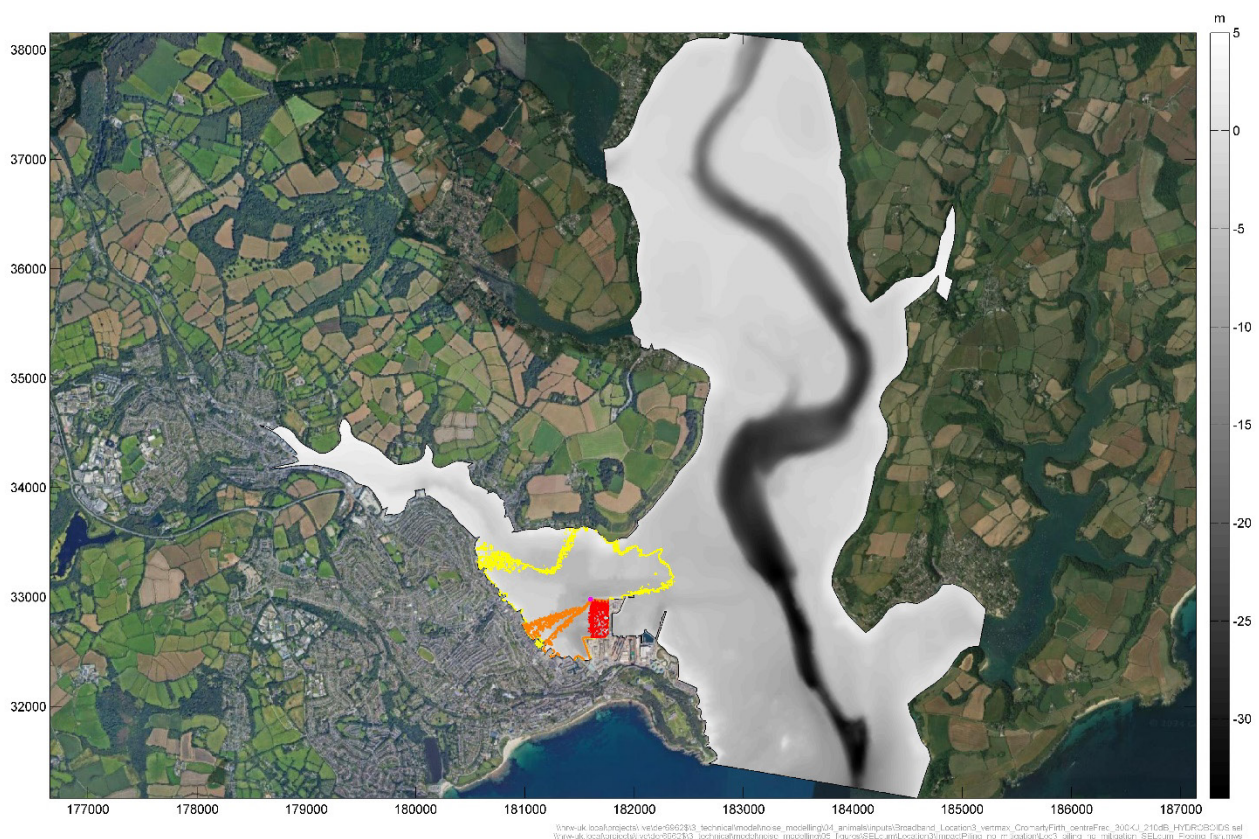
Figure 7.31: Predicted SEL_{cum} impact footprint for fleeing fish for percussive piling, with a soft start procedure, at the Queen's Wharf (Location 3)
