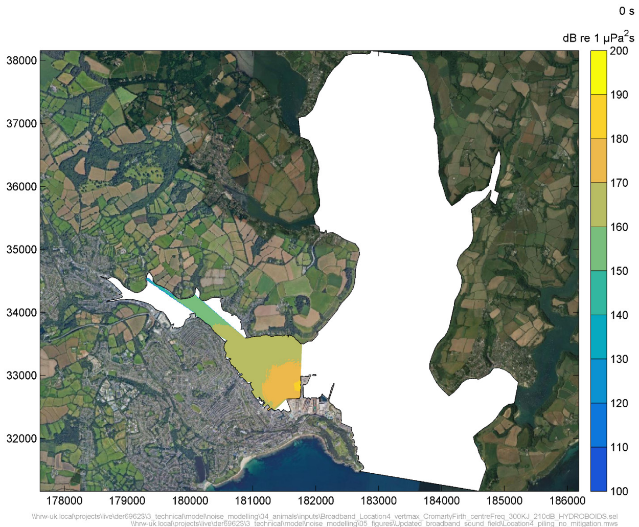
Figure 7.43: Predicted single strike SEL sound field for percussive piling at Location 4
