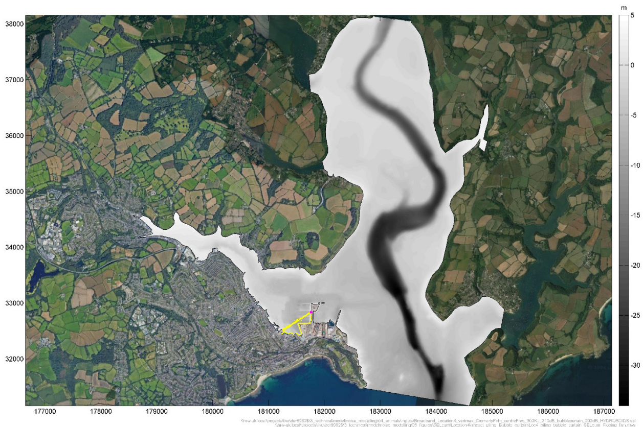
Figure 7.56: Predicted SEL cum impact footprint for fleeing fish for percussive piling, with a soft start procedure and bubble curtain, at the FLOW Deck (Location 4)
