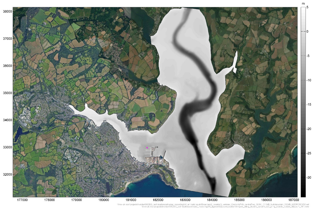
Figure A.29: Predicted SEL cum impact footprint for the for high frequency cetaceans for pile driving with a bubble curtain at Queen's Wharf (Location 3)
