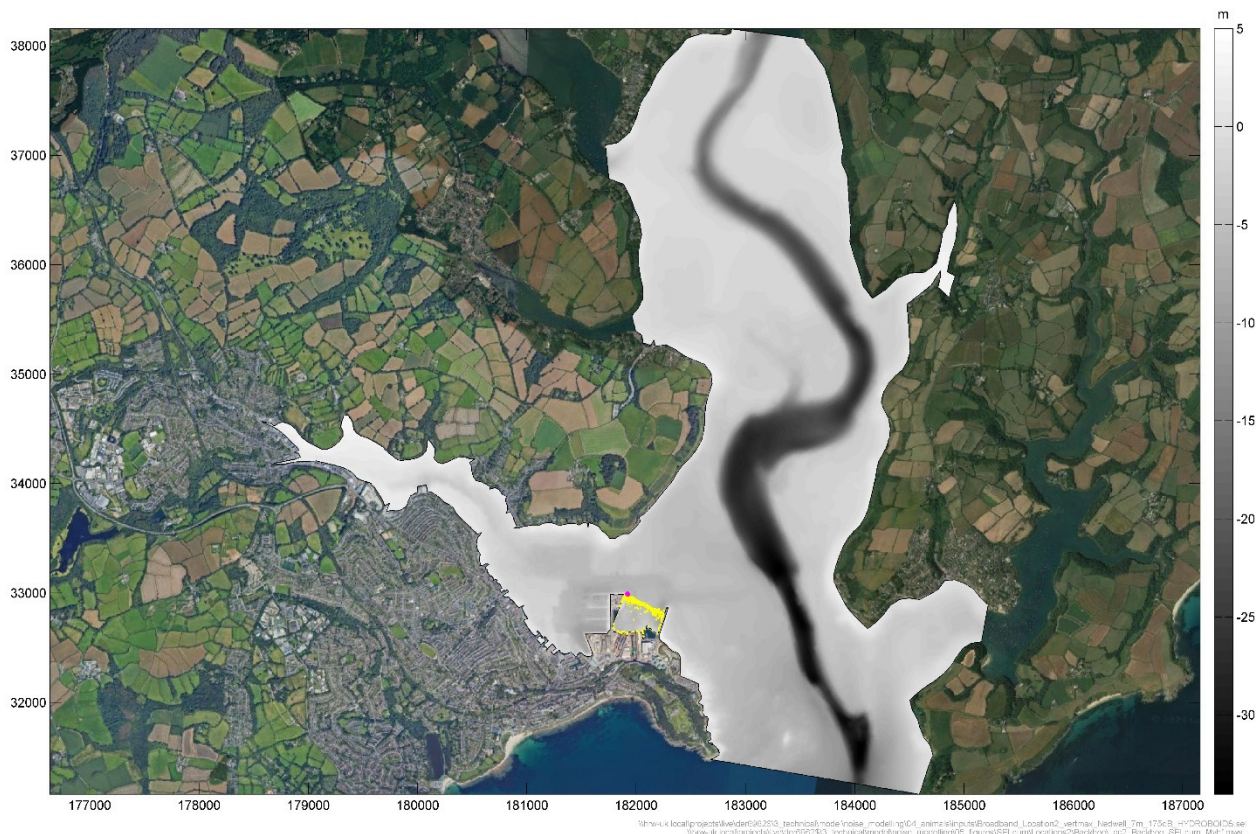
Figure 7.10: Predicted SEL cum impact footprint for the very high frequency cetacean hearing group for dredging with a backhoe at the Western Wharf (Location 2)
