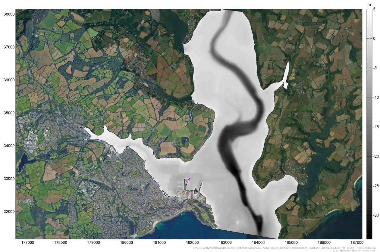
Figure A.10: Predicted SEL cum impact footprint for the for pinnipeds for dredging at Western Wharf (Location 2)
