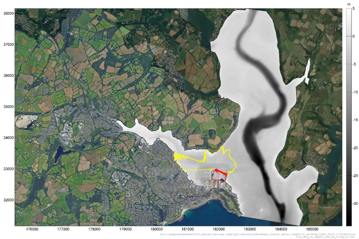
Figure A.15: Predicted SELcum impact footprint for the for fleeing fish for pile driving, at the Western Wharf (Location 2)
